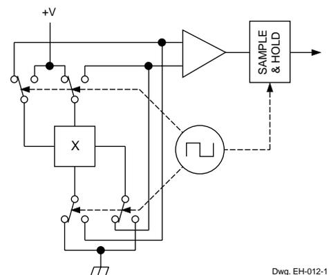
Electronically Rotated Sensor to Cancel Effects of Strain
